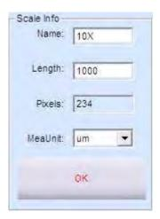
6. Click [OK] to confirm the calibration. The new calibration file named "10X" is created in the [Calibrate Table].
