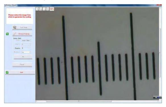
4. Click [Distance scaling] and move the cursor to the slide image, draw a line to get the reference length.
