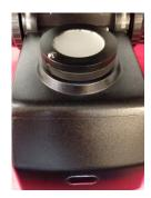
This component is comprised of two flanges; a semi-permanent mounting flange and a swing-in diffuser. The lower flange has a four-tooth bayonet arrangement. Placing it on the light port as shown below will allow it to seat down onto the light port.
