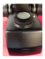
Next the assembly is rotated 45 degrees. This will engage the bayonet teeth. When correctly installed, the thumb screw on the lower flange should face 3 o'clock. Lightly tighten the thumb screw.
