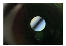
8. Slightly rotate the Polarizer (located on the light port)—seeking to make the shear line as dark as possible.
