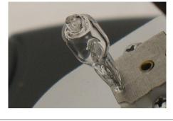
Replacing the Halogen Lamp in the Bottom Illuminator (Fig. 11)
