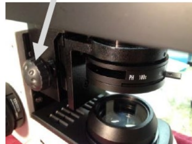
Condenser Height Adjustment Knob
