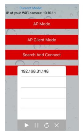
When several devices are connected to WiFi camera through "AP client mode", several search results will be available. The IP address in the example is the WiFi camera address connected to the router. Click this address and the software can connect different cameras through the router. Note: if the search time for the relevant IP address is beyond 76 seconds,
