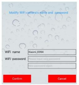
Step 3: Exit the software, go to the device wireless local area network and connect the camera. The camera name is the newly modified WiFi name and the password is the modified one. Reenter the software to use the camera with the new WiFi name.
