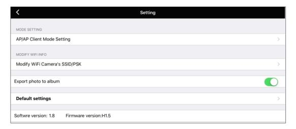
Step 2: Select "modify WiFi camera SSID/PSK" to enter modification interface. Please complete the name and code setup according to hint. Note: the code requires no fewer than 8 characters.
