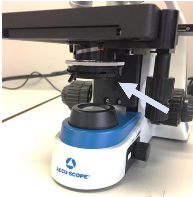
Darkfield stop in closed position
