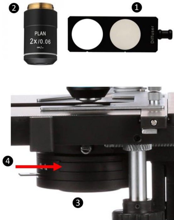
Slider blank (red arrow) shown insert into filter slider slot of 3000-LED microscope.
