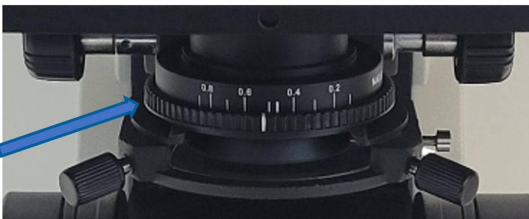
Condenser Aperture Diaphragm Adjustment
