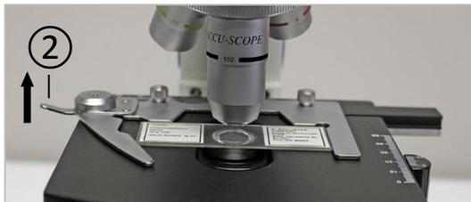
Rotate the X and Y-axis knobs ③ to move the slide into position.
