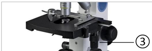
Place a specimen slide on the center of the stage.
